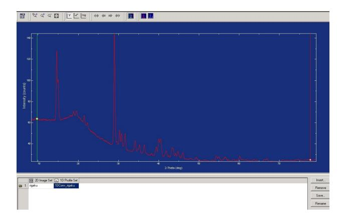
You can improve the 1-dimensional pattern by using a 'blank' for background correction. A blank is created by using an empty loop and running the same experimental conditions as the sample. You can correct background by using the 'Correct Background' feature listed under the Load instruction. You will be prompted for the name of the background file.
