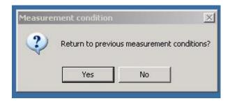
If you answer yes, you experimental setup will be the same as the one run just before you. If you answer no, the default experimental conditions will be set. The default setup uses an incorrect setting for KV and mA, which should be set to 40/40.
