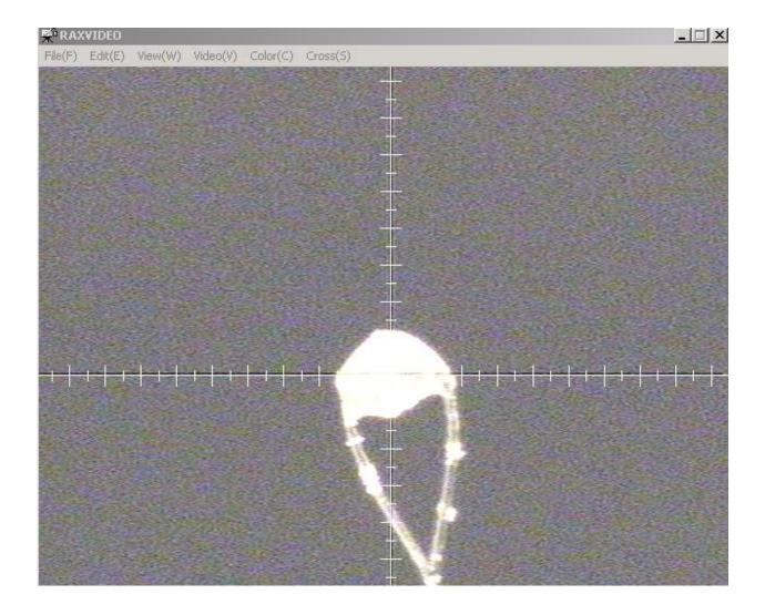
When you have aligned the sample, you can setup the data collection parameters. Typically, for a loose powder, you will leave omega at  $70^{\circ}$  and chi at  $0^{\circ}$  and you will rotate phi continuously. A good trial setup would be to collect data for 600 seconds while continuously rotating phi with the generator set to 40 KV and 40 mA.
