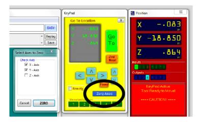
10. You are now ready to zero the Z axis. If you are using the vacuum hold down, open and/or close the appropriate valves and turn the vacuum on using the switch to the left of the computer.
