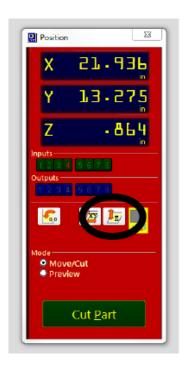
13. Click "OK" when the spindle is above the plate, and allow the machine to zero the Z axis. Once the machine is zeroed, put away the Z Zero Plate and alligator clip and click "OK" in the dialogue window that appear on screen.
