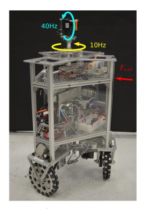
Fig. 1. **Trikey** with 360° LIDAR and torque sensors on its drivetrain. The laser ray from the LIDAR rotates with 10Hz horizontally, 40Hz vertically. Also, external forces applied to the system are detected the torque sensors in its drivetrain.
