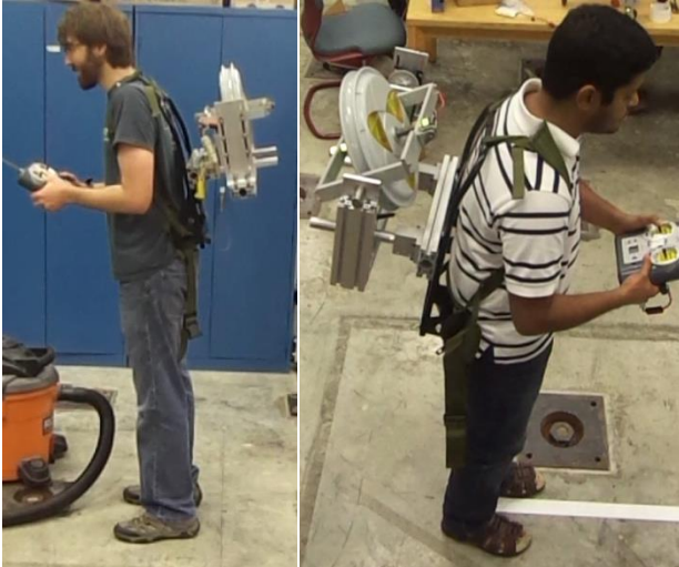
Figure 12. Backpack mounting of the gyroscope on two human-subjects
