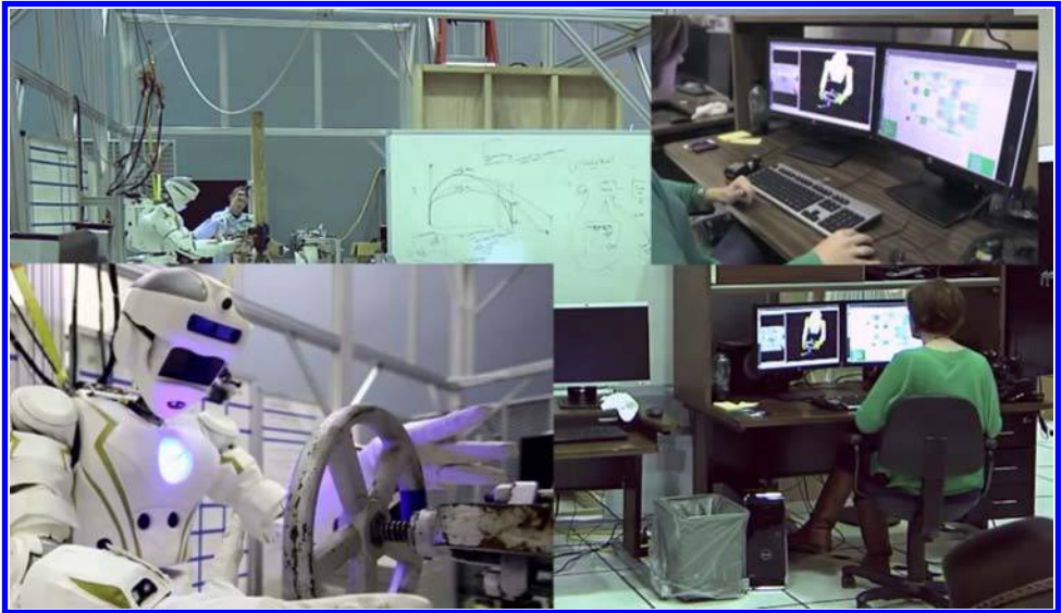
Fig. 17. This figure shows Valkyrie's upper body being controlled by an early version of ControlIt!. Using a compound task consisting of Cartesian position and orientation tasks for each hand, and a flat contact constraint for the torso, a human operator uses Valkyrie to turn an industrial valve. Parameter binding is used to integrate ControlIt! with the operator's command and visualization applications.
