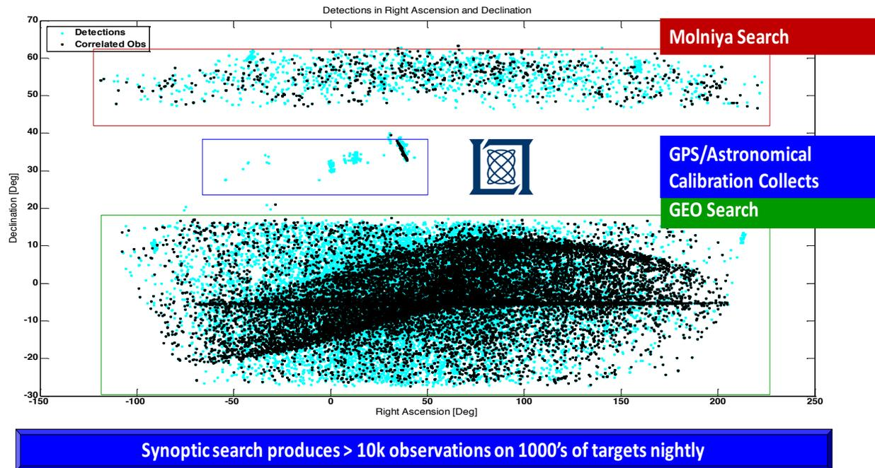
**Figure 1. A Single Night's Worth of Resident Space Object (RSO Detections (for various orbital regions) from the U.S. Space Surveillance Telescope (SST) in New Mexico. Detections (dots) that are Black are those believed to be from known (cataloged) RSOs. All else (Cyan) are Detectable but Untrackable RSOs.**
