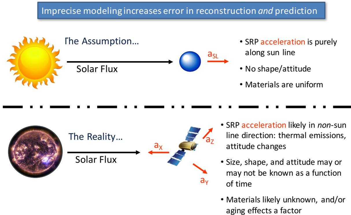
**Figure 2. Difference between the motion experienced by a spherical (cannonball-like) space object and a satellite with realistic size, shape, orientation, and material properties. For the sphere, the acceleration due to the sun's effects are unidirectional. In reality, our tracking data informs us that objects experience accelerations due to the Sun's effects in 3-dimensional space (multi-directional).**
