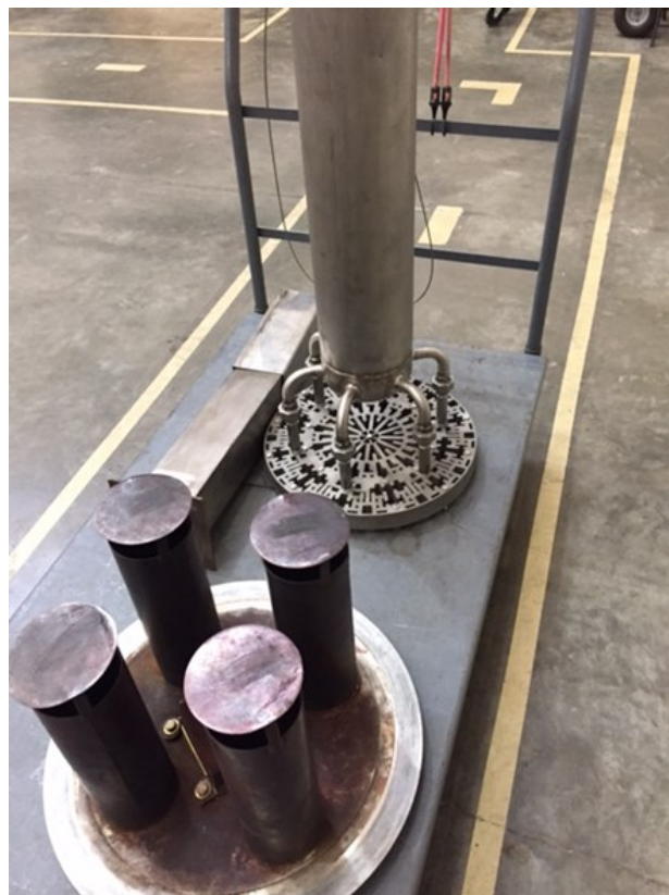
Stainless Steel Fractal Liquid Distributor and Chimney Tray Used in the Distillation Study
