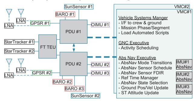
Figure 1. Orion Absolute Navigation Architecture - General View
