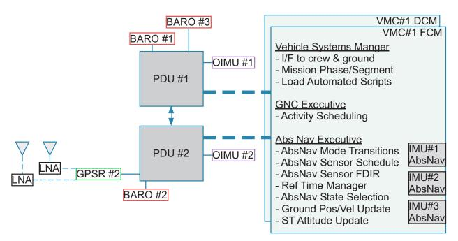
Figure 2. Orion Absolute Navigation Architecture for EFT-1
