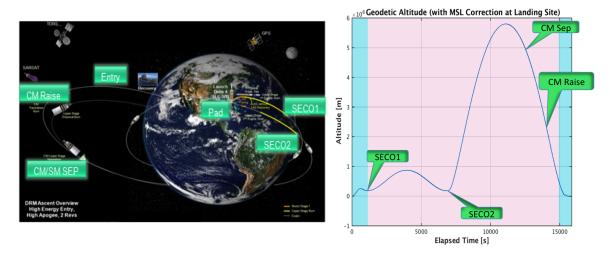
Figure 1. Orion EFT-1 Trajectory Overview and Flight Altitude Profile
