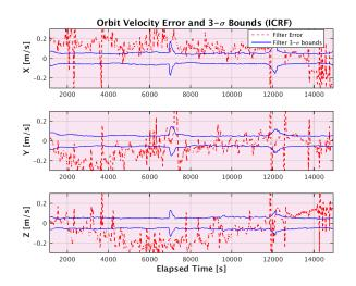
Figure 13. Orbit On-board Filter Velocity Uncertainty
