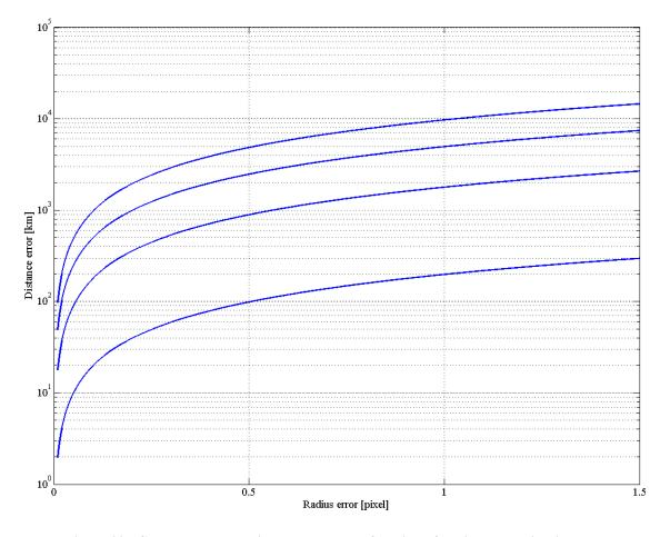
Figure 20. Calculated Moon distance error as a function of radius determination error
