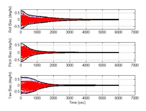
Figure 2. Gyro bias estimation error of qEKF
