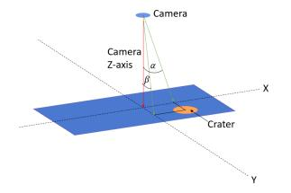
Figure 3: Camera Axes and Bearing Angles
