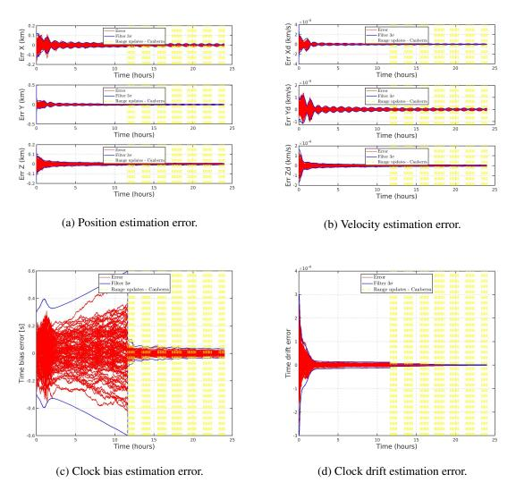
Figure 6: Estimation errors with one-way ranging measurements from Canberra station only.
