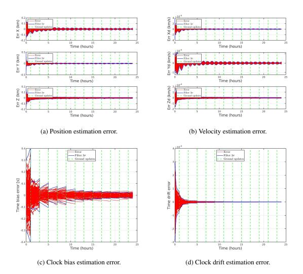
Figure 7: Estimation errors with craters measurements and position ground updates.
