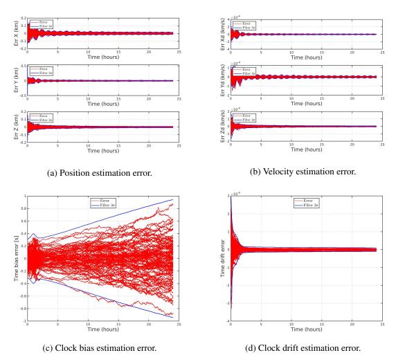
Figure 2: Estimation errors with craters measurements only.
