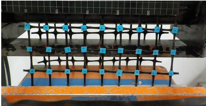
Figure 3.6 - Disposition of the markers on the unconfined portion of the geosynthetic.
