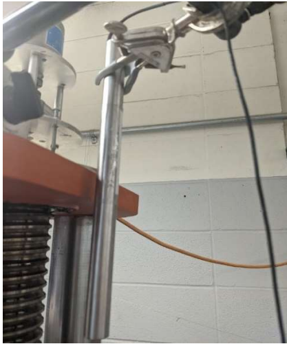
Figure 3.3 - LVDT used to check the displacement rate of the loading frame.
