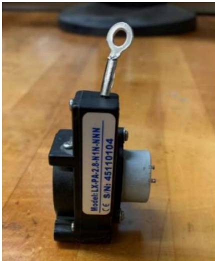
Figure 3.4 - Close view of one of the LPs used to measure displacement during the SGI test.
