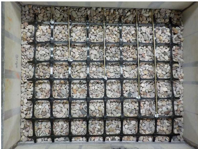
Figure 3.8 - Top view of the box after the first two layers and the geosynthetic are placed.
