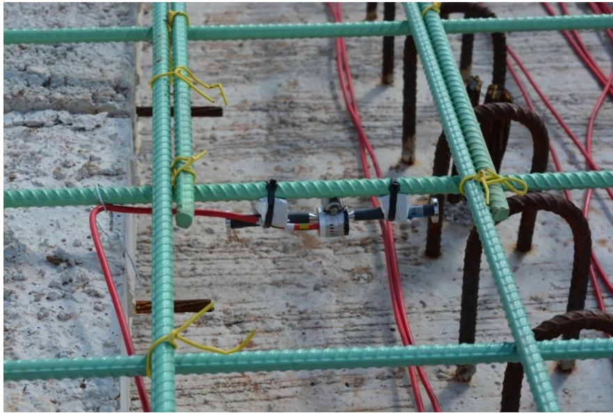
Figure B. 14: GK-4200L as installed on the deck, perpendicular to the direction of the bridge, March 2020
