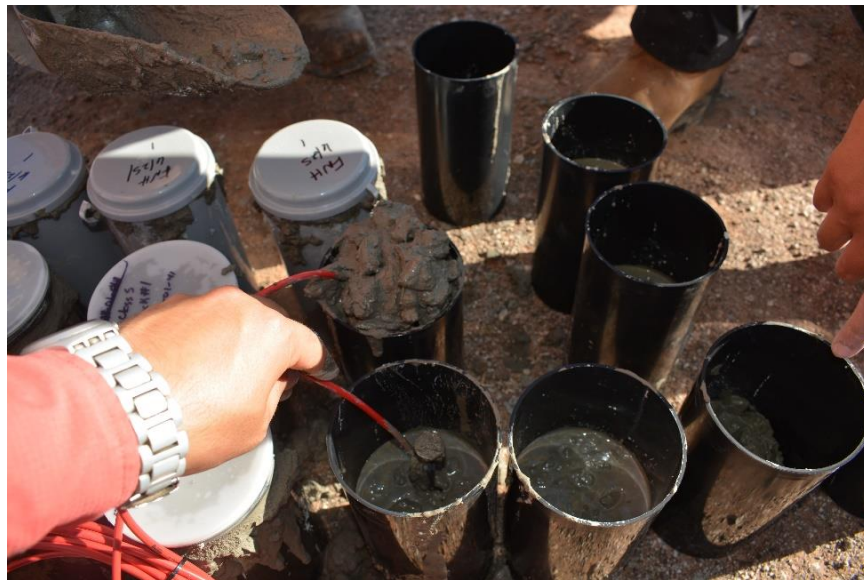
Figure B. 45: Instrumented concrete sample cylinders
