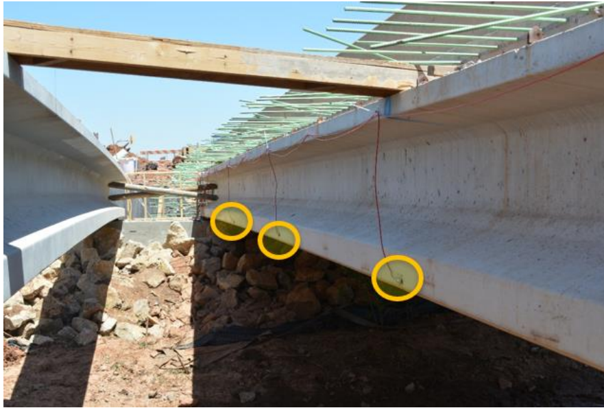
Figure B. 40: Mounted miniature strain gauges on the bottom flange of the middle girder
