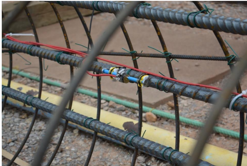
Figure B. 27: Strain gauges attached to the long. rebars of drilled shafts
