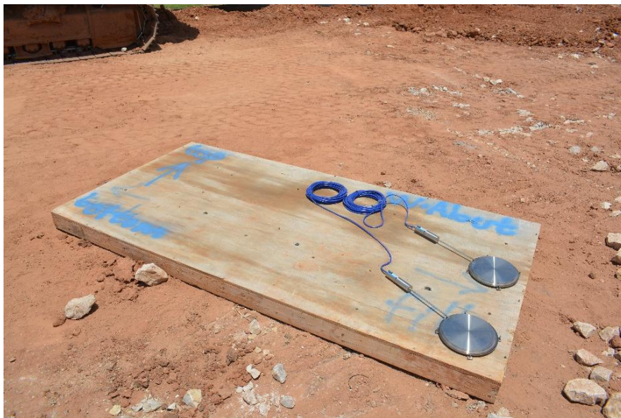
Figure B. 42: A pair of earth pressure cells mounted on the back of the form intended for the west abutment wall
