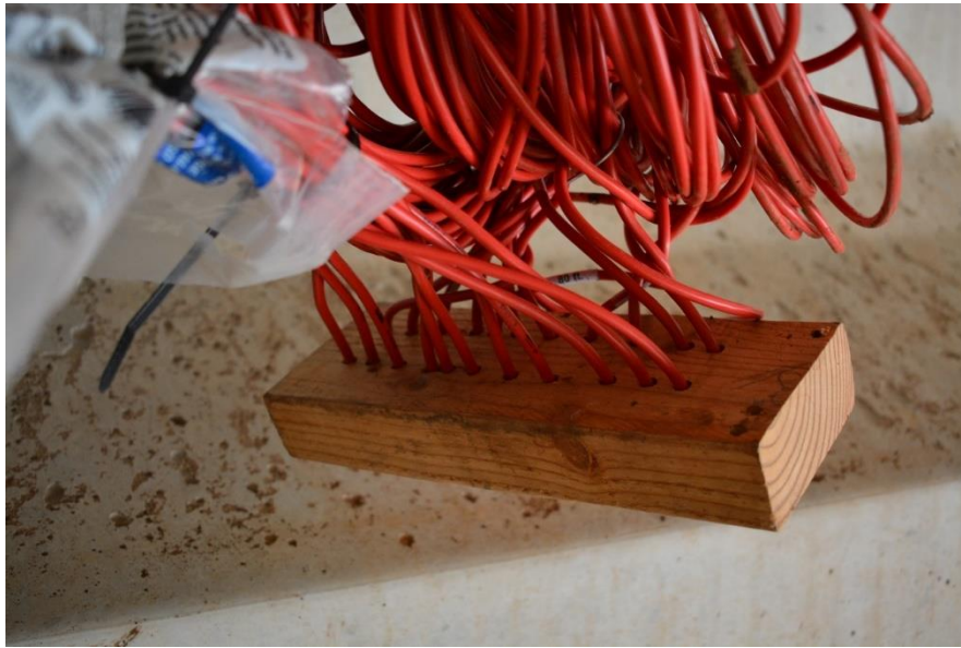
Figure B. 18: Predrilled block of wood used to help keep track of the cables coming from embedded strain gauges
