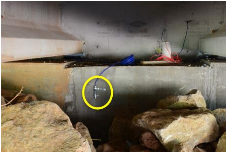
Figure B. 54: Creekside piezometer installed on the abutment cap
