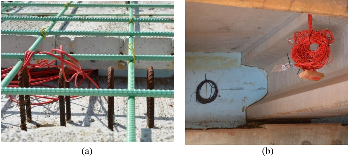
Figure B. 17: Installation of strain gauges: (a) cables of the strain gauges were routed through a small gap between the foam boards to underneath the bridge, and (b) coiled up wires coming from the strain gauges (red) and earth pressure cell (blue).
