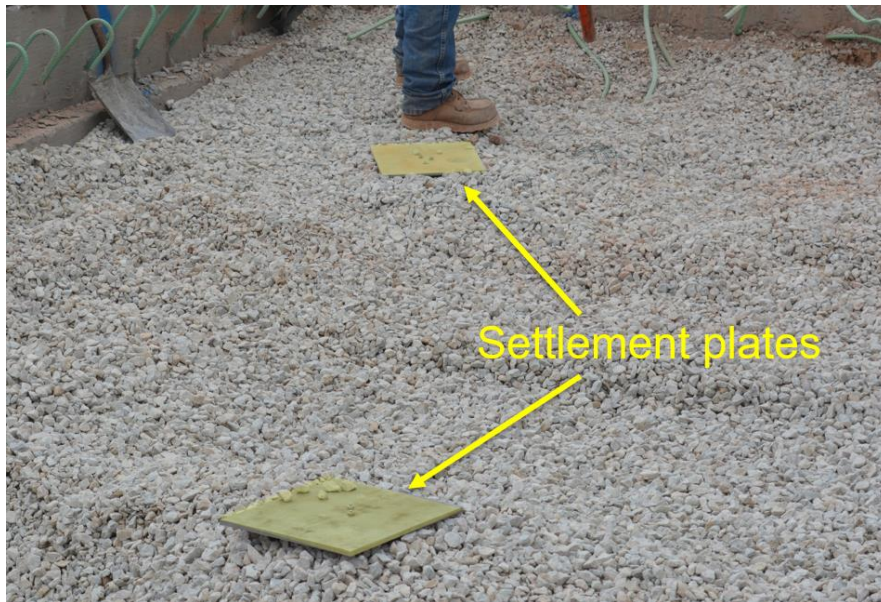
Figure B. 49: Stainless steel plates attached to the top flange of the settlement sensors
