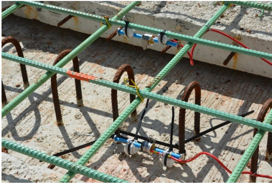
Figure B. 15: A pair of GK-4200 strain gauges installed on the deck during phase 1 of the construction
