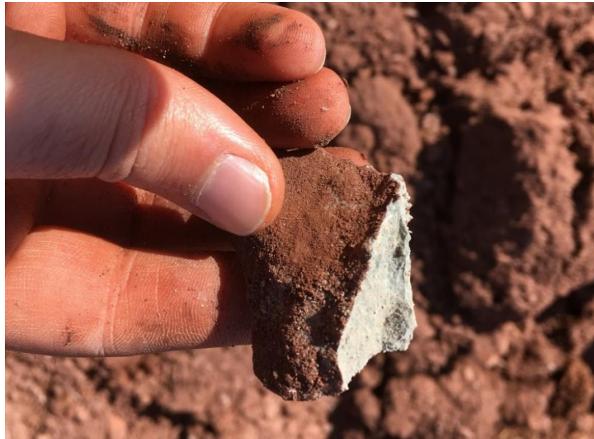
Figure B. 8: Gray shale covered with powdery red dirt recovered from 8 m depth
