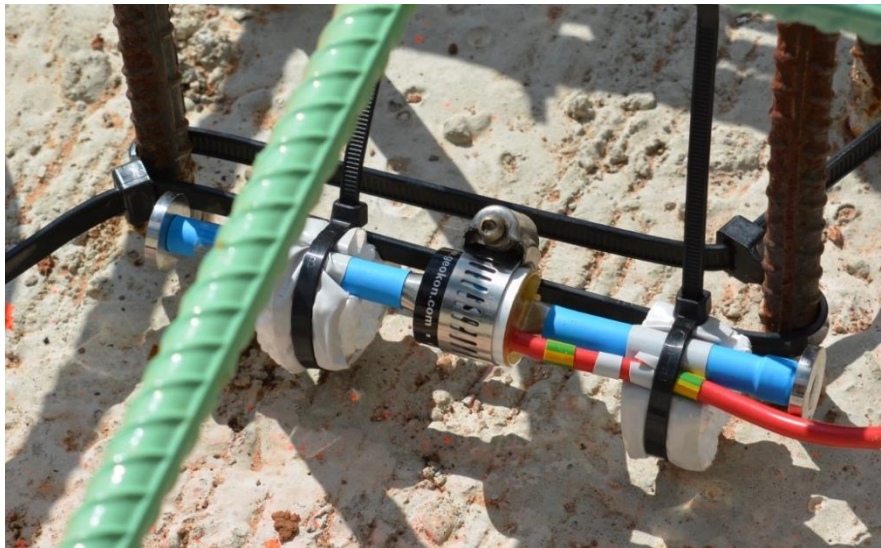
Figure B. 16: Identification of strain gauges using colored tapes as binary ID code
