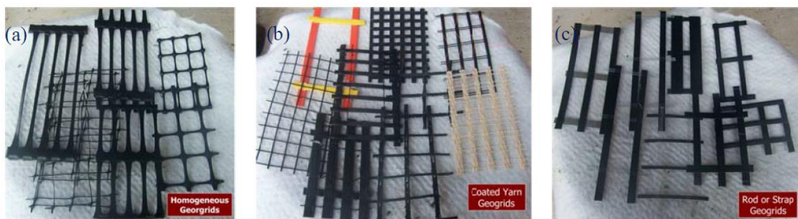
Figure A.1 Various types of Geogrids: (a) Homogenous; (b) Coated Yarn; (c) Welded;
