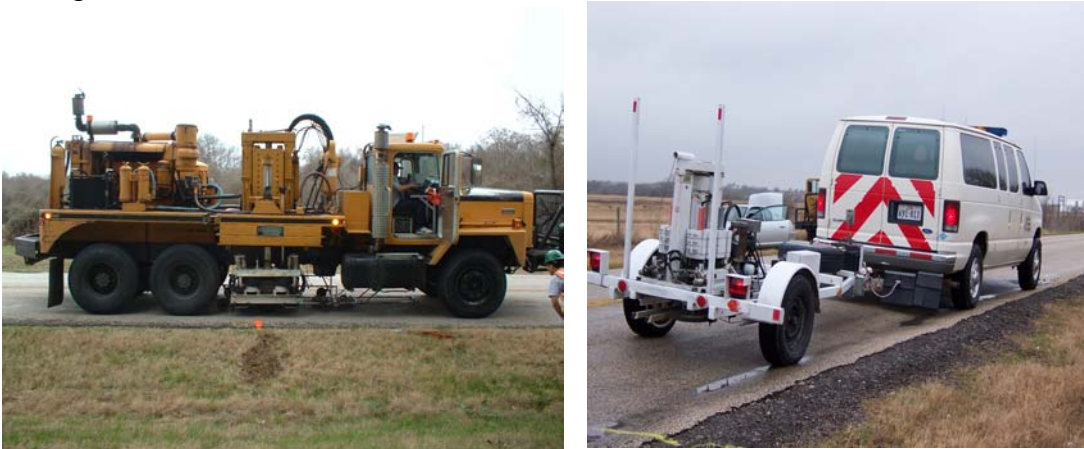
Fig 3: RDD and FWD testing done at pavement on a Farm to Market Road
