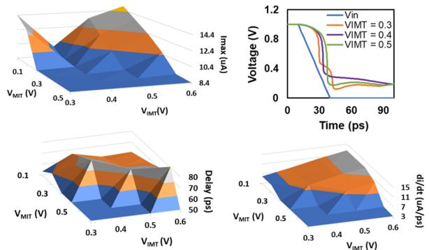
**Fig. 6 Variation of  $I_{MAX}$ ,  $di/dt$  and delay with the PTM device parameters  $V_{IMT}$  and  $V_{MIT}$**
