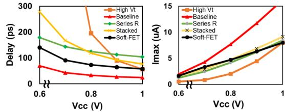
**Fig. 5 Comparison of Soft-FET with various CMOS topologies for peak switching current reduction**
