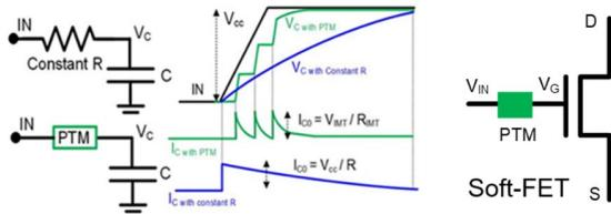
**Fig. 3 Soft charging using phase transition materials**
