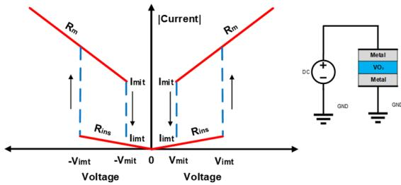
**Fig. 2 Phase Transition Material: I-V characteristics**
