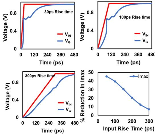
**Fig. 9 Effect of input slew rate on the PTM switching behavior**
