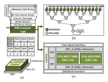
Fig. 7. (a) Bank-level PIM organization, (b) Newton compute logic, and (c) HBM-PIM compute unit.
