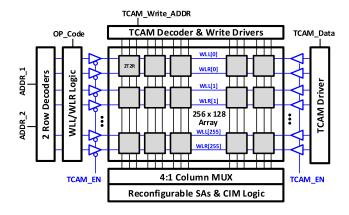
Fig. 12. 2T2R ReRAM macro for versatile PIM functions [49].
