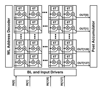
Fig. 4. Digital SRAM-based processing-in-memory macro [18].
