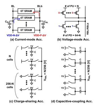
Fig. 3. SRAM-based accumulation mode.
