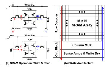
Fig. 1. SRAM background: (a) Operation; and (b) Architecture.
