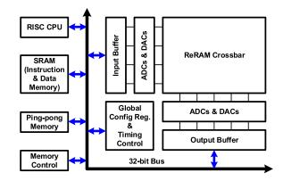
Fig. 11. Block diagram of ReRAM coprocessor [46].
