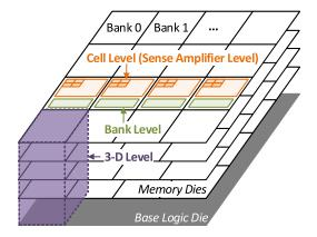
Fig. 5. Different levels of DRAM PIM architectures.
