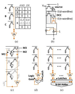
Fig. 6. (a) AMBIT TRA, (b) AMBIT DCC, (c) DRISA 3T1C-NOR, (d) DRISA 1T1C-NOR/MIX, and (e) DRISA 1T1C-ADDER.
