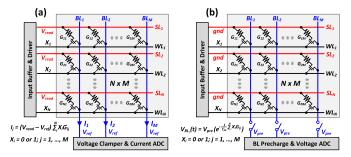
Fig. 9. ReRAM-based PIM architectures for MAC based on: (a) Currentmode sensing and (b) Voltage-mode sensing.
