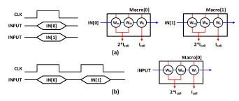
Fig. 10. Multiplication of 2-bit inputs and 2-bit weights in digital ReRAMbased PIM: (a) One cycle and multiple macros and (b) Multiple cycles and one macro.
