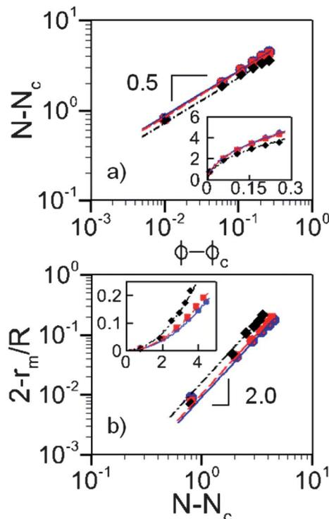
**Fig. 3** (Color online) Simulation results (symbols) and corresponding models for  $N - N_c$ (a) and  $2 - r_m/R$ (b). Lines: fits with scaling laws using constants  $K_r = 0.0091, 0.0105, 0.016$  and  $K_N = 8.67, 8.49, 7.31$  for Hertz (circles), compressed emulsions (squares) and Mooney-Rivlin materials (diamonds), respectively. Insets: linear scale.
