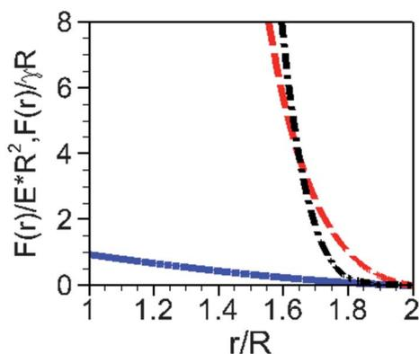
**Fig. 2** (Color Online) Elastic Repulsion forces for hertz potential (solid lines), compressed emulsion potential (dashed) and Mooney-Rivlin material potential (dash-dot).
