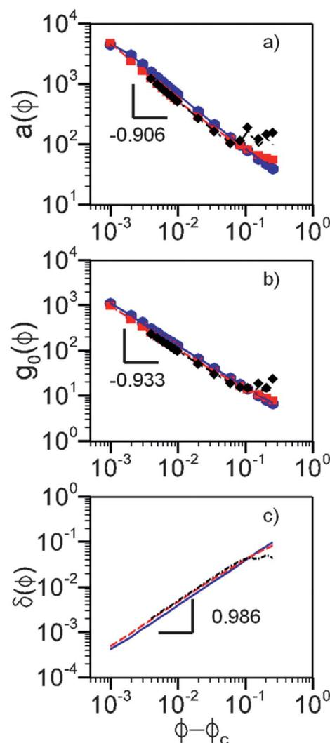
**Fig. 6** (Color online) Computational (symbol) and analytic (lines) predictions of  $a(\phi)$  and peak and width of  $g(r)$  for different volume fractions. (Circles/solid lines – Hertz potential, square/dashed lines – compressed emulsion potential, diamonds/dashed-dotted lines – Mooney-Rivlin potential).
