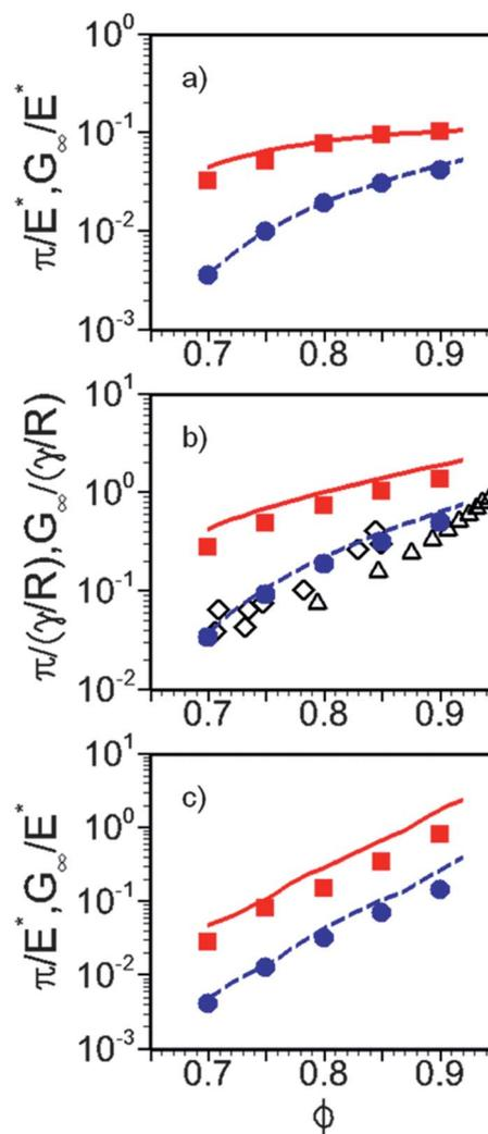
**Fig. 8** (Color online) Comparison of theoretical predictions (lines) of elastic properties for a) hertz potential, b) compressed emulsion potential and c) Mooney-Rivlin material potential with computer simulations (circles – osmotic pressure and squares – high frequency modulus) and experiments on osmotic pressure of compressed emulsions (diamond)<sup>10</sup> and foams (triangle).<sup>37</sup> Upper lines: high frequency elastic modulus and lower lines: osmotic pressure.
