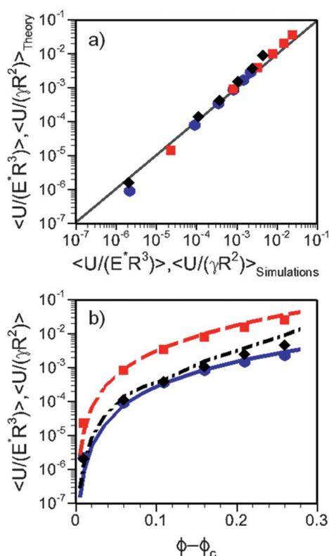
**Fig. 4** (Color online) a) Comparison of theoretical predictions (lines) of average elastic energy with simulation results (symbols). b) Variation of average energy with volume fraction for Hertz (circles), compressed emulsions (squares) and Mooney-Rivlin materials (diamonds).
