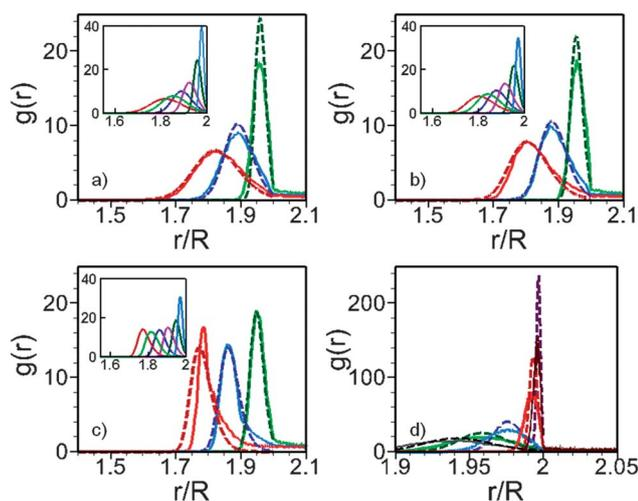
**Fig. 5** (Color online) Comparison of theoretical predictions from eqn (5) (dashed lines) of  $g(r)$  with computer simulations (solid lines) for a) Hertz potential, b) Compressed emulsions and c) Mooney-Rivlin material. Right to left in a), b) and c): volume fraction = 0.7, 0.8 and 0.9. Insets: Theoretical predictions for volume fractions 0.675, 0.7, 0.75, 0.8, 0.85 and 0.9 (right to left). d) Hertz potential – volume fractions 0.645, 0.65, 0.675, 0.7, 0.725 (right to left).
