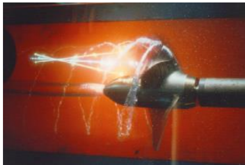
Figure 1. A cavitating propeller with developed tip vortex cavities and a hub-vortex cavity originating from the blade tip and the hub. With permission granted by Professor Spyros A. Kinnas.
