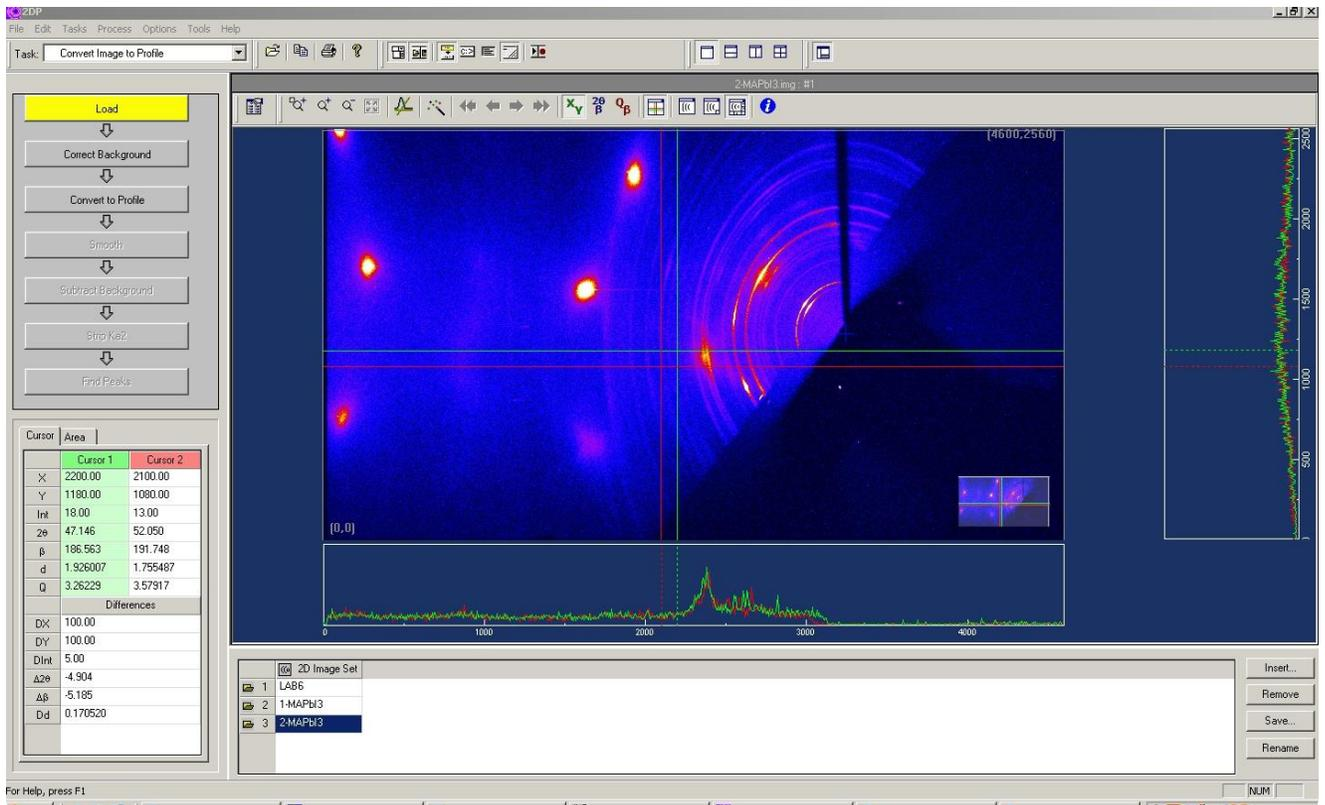
The slope image is due to the chi angle setting. The large reflections are single crystal reflections from the substrate. Select the Convert to Profile menu item to generate a 1-dimensional pattern from the 2-dimensional image collected.
