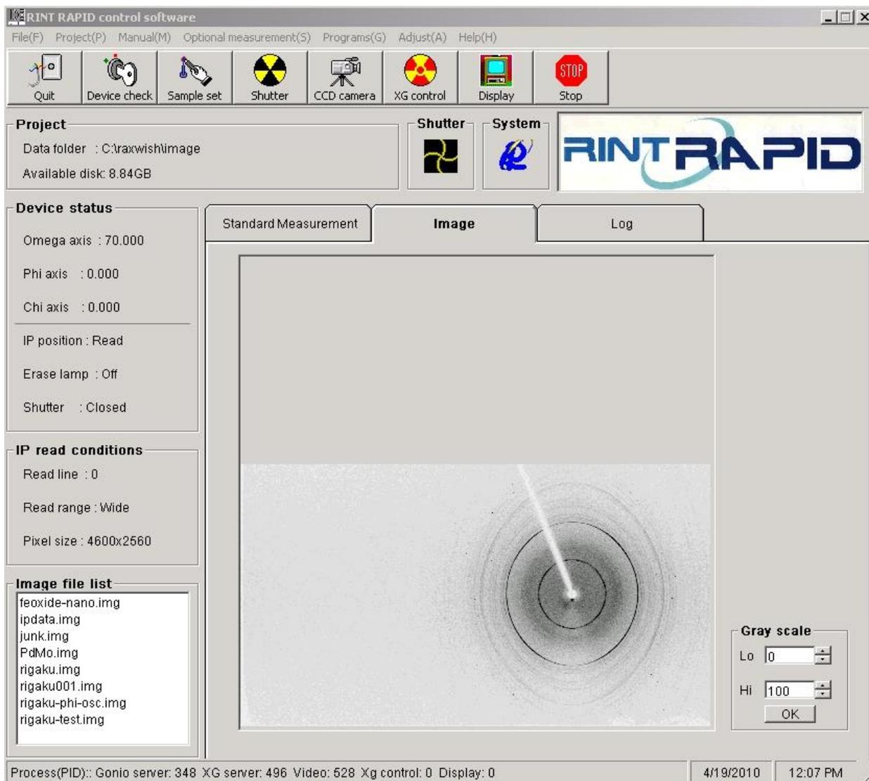
The 2D image can be converted into a 1D image suitable for data analysis in Jade or Bruker-
