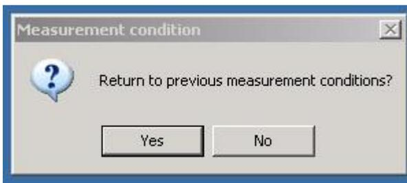
If you answer yes, your experimental setup will be the same as the one run just before you. If you answer no, the default experimental conditions will be set. The default setup uses an incorrect setting for KV and mA, which should be set to 40/40.
