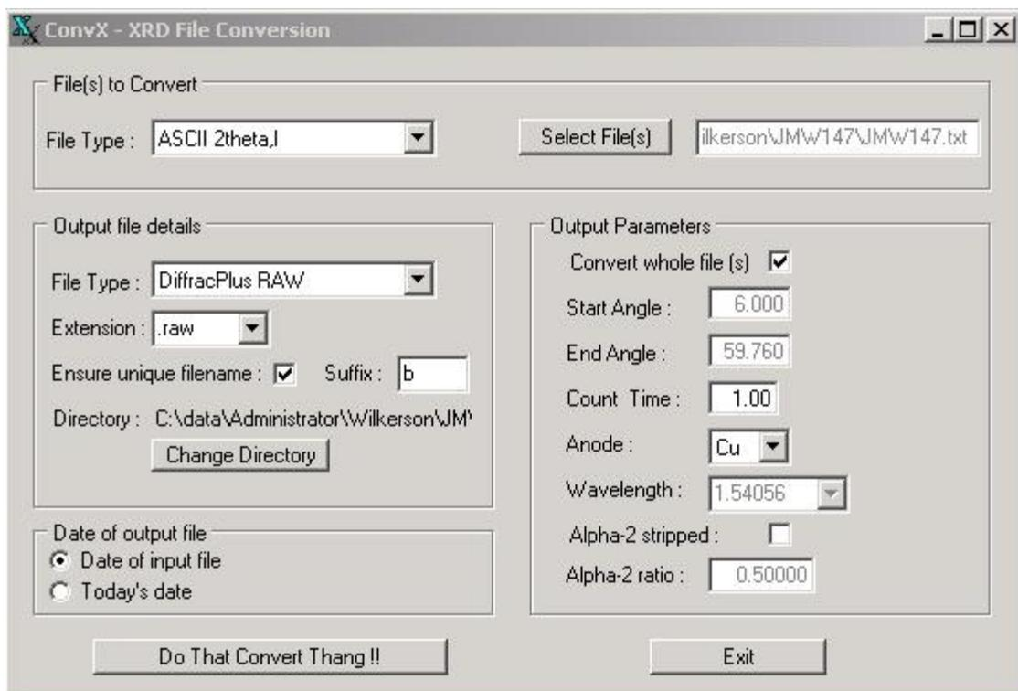
The default file type for ASCII 2theta, I is .dat. You will have to select the appropriate .txt file. The output file type is DiffracPlus Raw. This is the Bruker format needed for Eval. Make sure the Anode type is set to Cu. The wavelength is set automatically. You can convert one or several files at once. The newly created .raw files will be stored in the same directory as the .txt files unless you have created a separate directory, which is recommended.
