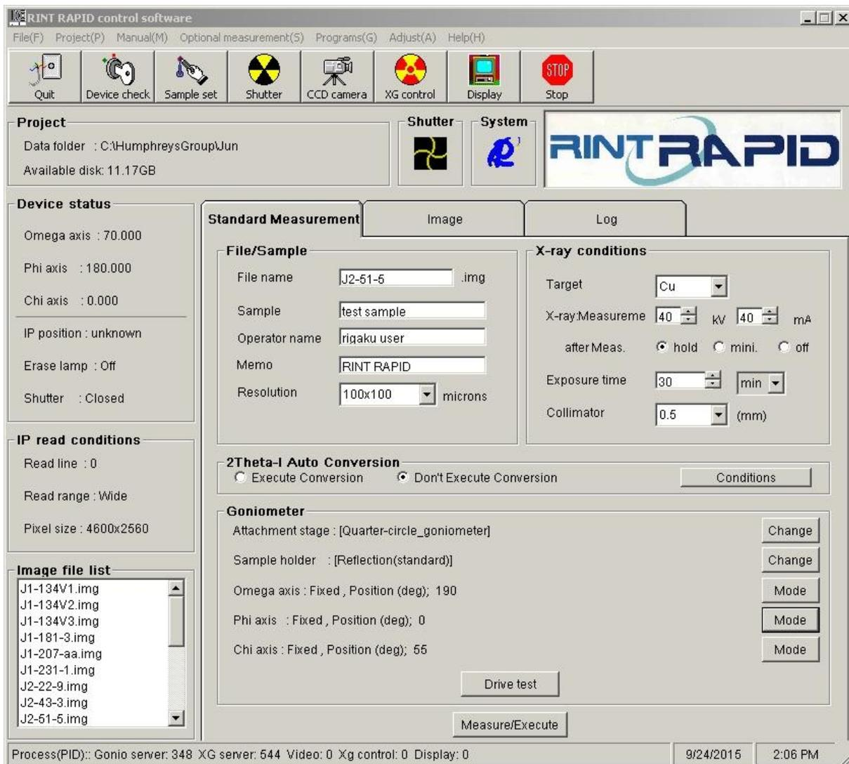
Hit Measure/Execute to start the data collection process. Be patient, the goniometer is slower than the others. In addition, the image plate detector may have to be erased before beginning. This process takes about 2 minutes as the detector is driven down to the read/erase heads in the bowels of the instrument. The yellow shutter open light will come on during data collection. When data is finished collecting, the image plate is driven to the read/erase heads and an image is created.
