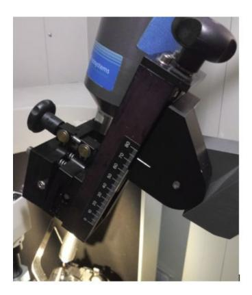
When you are finished collecting data, raise the nozzle out of the way for the next user. You should shut down the Cryostream as well. Don't simply turn it off. Use the CryoPad controller and select END in the cooling Phase and click on Execute Now. Finally, turn off the AD51 controller. It will finish on its own. You are done.
