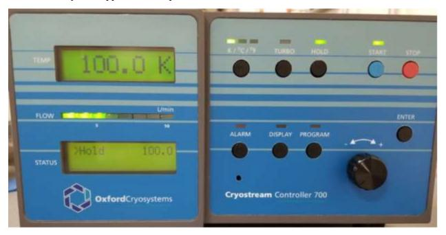
Check that there is some liquid N2 in the 60L Dewar. To check, lift the transfer line up enough to place a meter stick into the opening. You will need at least 10 cm of liquid N2 for several hours of operation, 25 cm for an overnight run. Use the 160L Dewar to fill it when needed.
