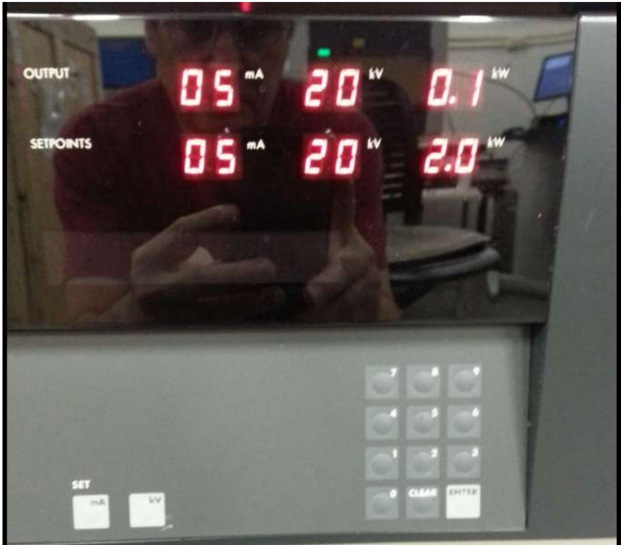
When increasing the power to the X-ray tube, always bring kV up first to its maximum setting of 50 kV and then mA to its maximum setting of 30 mA. When decreasing the power, bring
