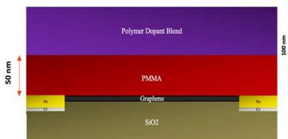
Fig 1. Cross-Section Schematic of the device structure. The graphene/PMMA layer is deposited on top of Au/Cr electrode followed by the dopant blend.
