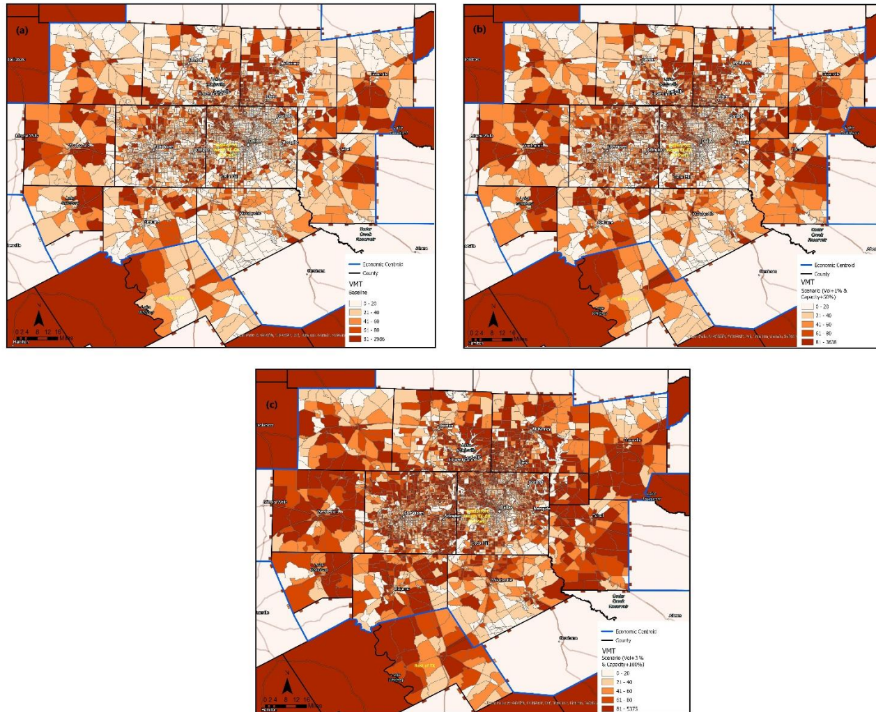
Figure 22. Personal VMT for the (a) Baseline, (b) a 50% increase in capacity with a 1% growth in traffic, and (c) a 100% increase in capacity with a 3% growth in traffic scenarios in Northern Texas
