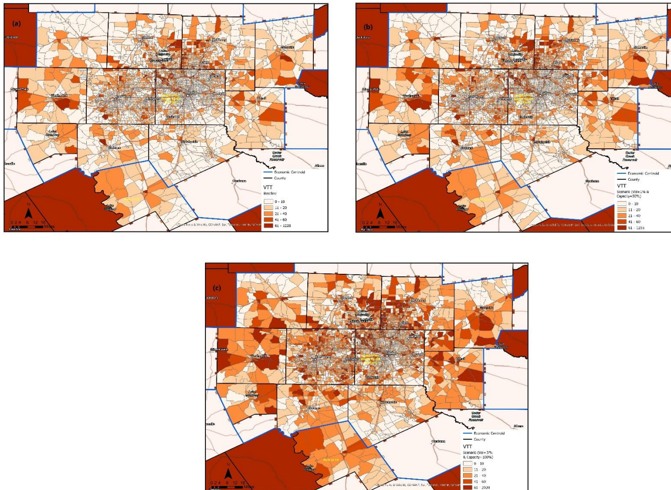
Figure 14. Personal Vehicle Travel Time for the (a) Baseline, (b) a 50% increase in capacity with a 1% growth in traffic, and (c) a 100% increase in capacity with a 3% growth in traffic scenarios in Northern Texas
