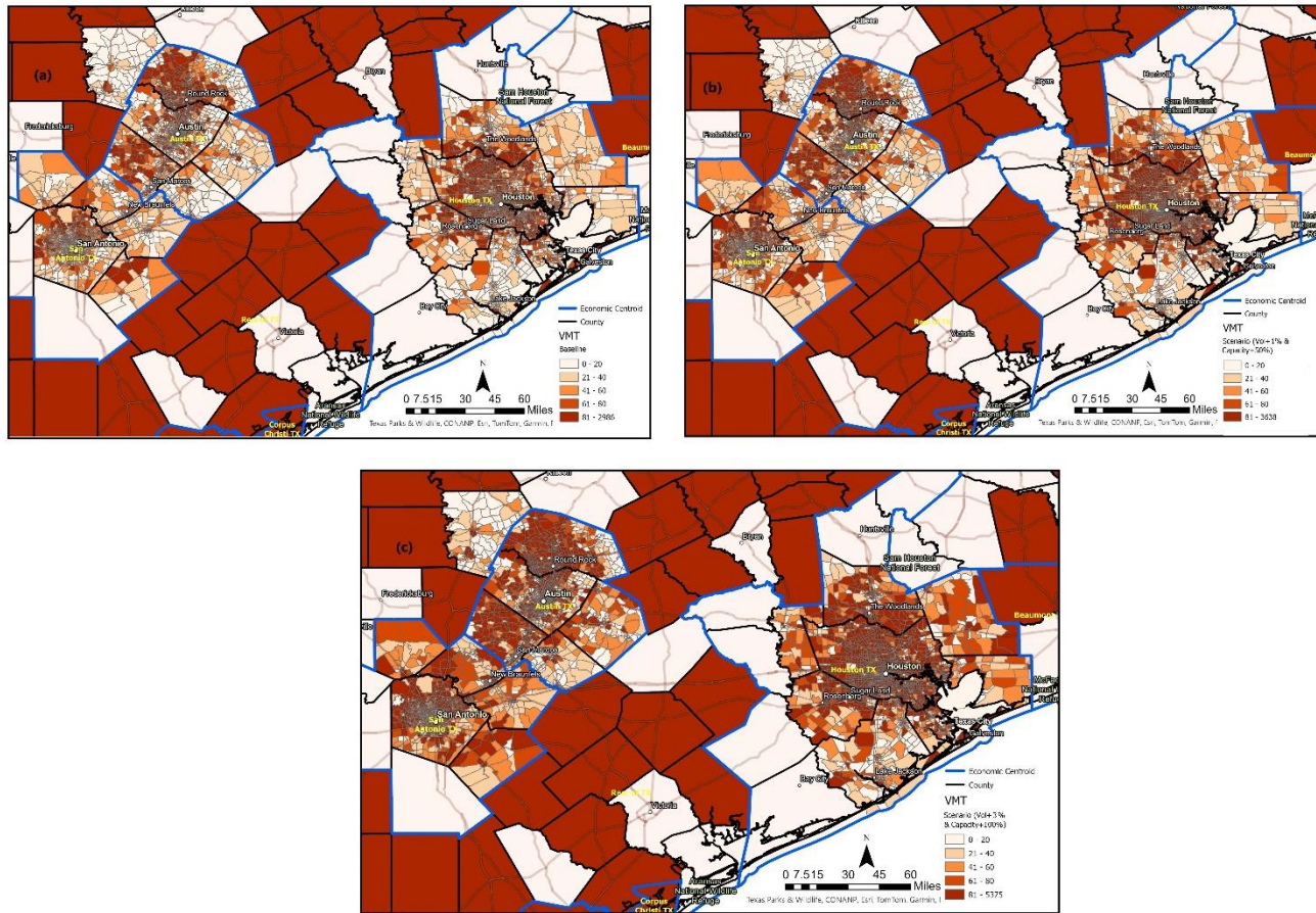
Figure 24. Personal VMT for the (a) Baseline, (b) a 50% increase in capacity with a 1% growth in traffic, and (c) a 100% increase in capacity with a 3% growth in traffic scenarios in Southern Texas
