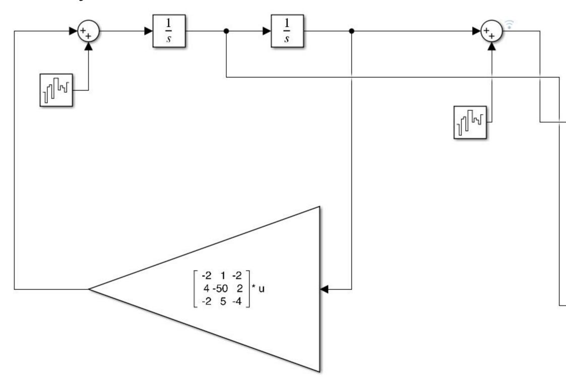
• The true dynamics were calculated by integrating the differential equations and adding measurement and process noise (chosen at this stage to give a noisy output that still approximately matched the output of the dynamics without noise)
