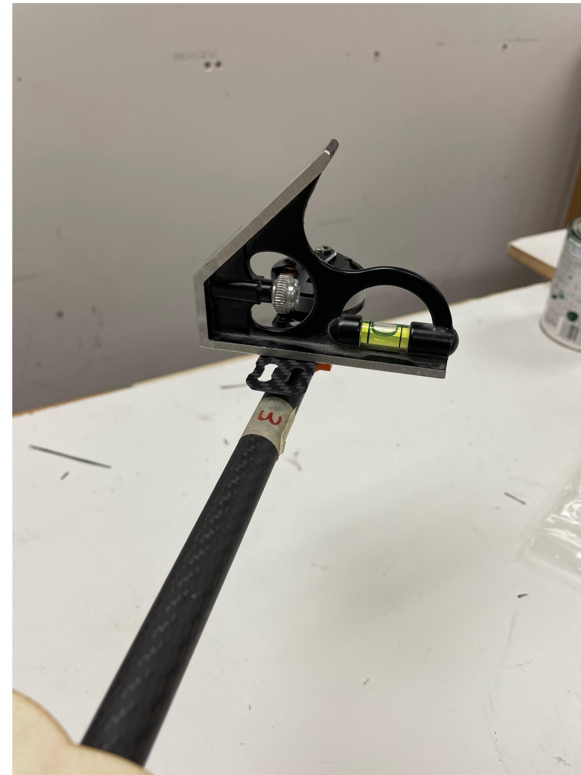
Level used to straighten motors
