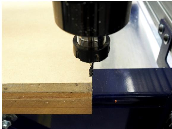
9. Once the spindle is in the proper X Y location, click the blue **Zero Axes** button on the **KeyPad** control window. A pop-up window will appear asking which axes you would like to zero. Select the X and Y boxes and click **Zero**.
