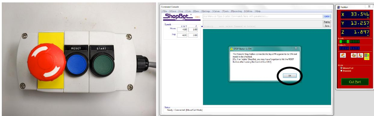
4. Open the **KeyPad** control window by pressing the yellow icon in the **Position** window.
