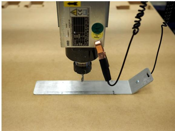
12. Close the **KeyPad** window and click the “Zero Z axis with Zero Plate” button.
