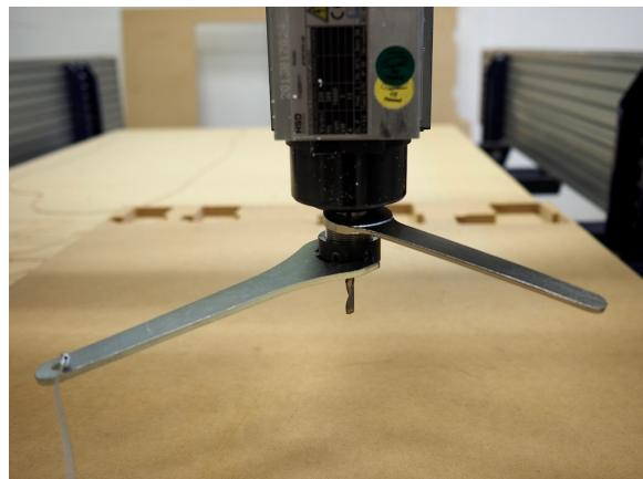
8. Using the **KeyPad** controls, move the spindle to the X Y zero location that corresponds to your toolpath file. This is generally the bottom right hand corner of your material.
