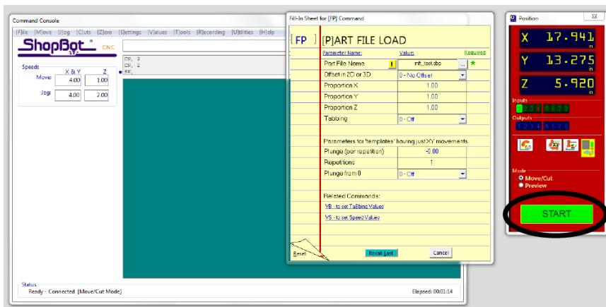
17. The program will ask if the Z axis is zeroed. Click “Yes” if you have zeroed the axis. If you have not, go back to step 11 and zero the Z axis using the Z Zero Plate.
