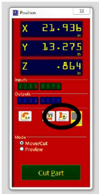
13. Click “OK” when the spindle is above the plate, and allow the machine to zero the Z axis. Once the machine is zeroed, put away the Z Zero Plate and alligator clip and click “OK” in the dialogue window that appear on screen.
