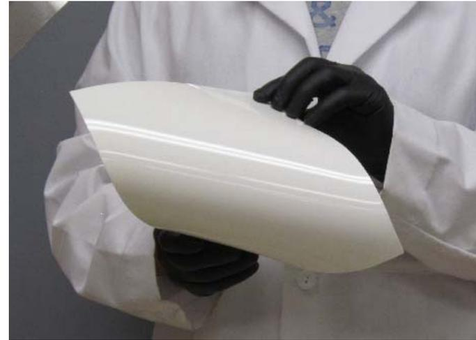
Photographs of a PEO/ $\text{Al}_2\text{O}_3$  (2/1 in weight) composite membrane ( $25 \times 20 \text{ cm}^2$ )
