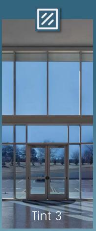
Visual light transmission: 6% Solar heat gain coefficient: 0.13
