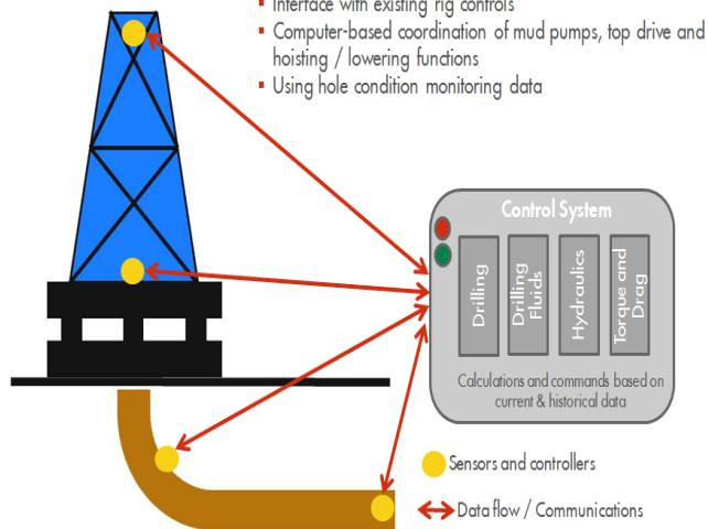
**Automate the drilling rig AND Control the rig from central location**
