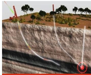
**"Manufacture" the wells by automated, truck-mounted rigs**
