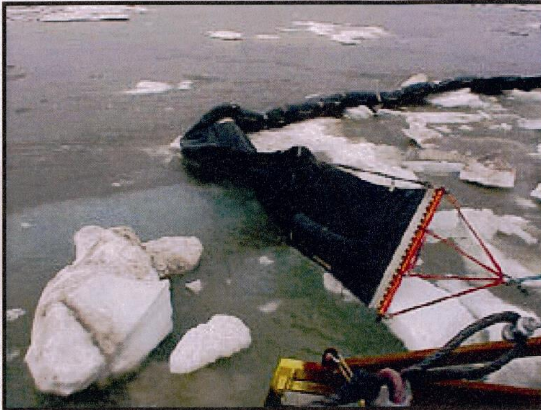
Figure 4. Photograph showing boom failure due to ice flowing under the boom.
