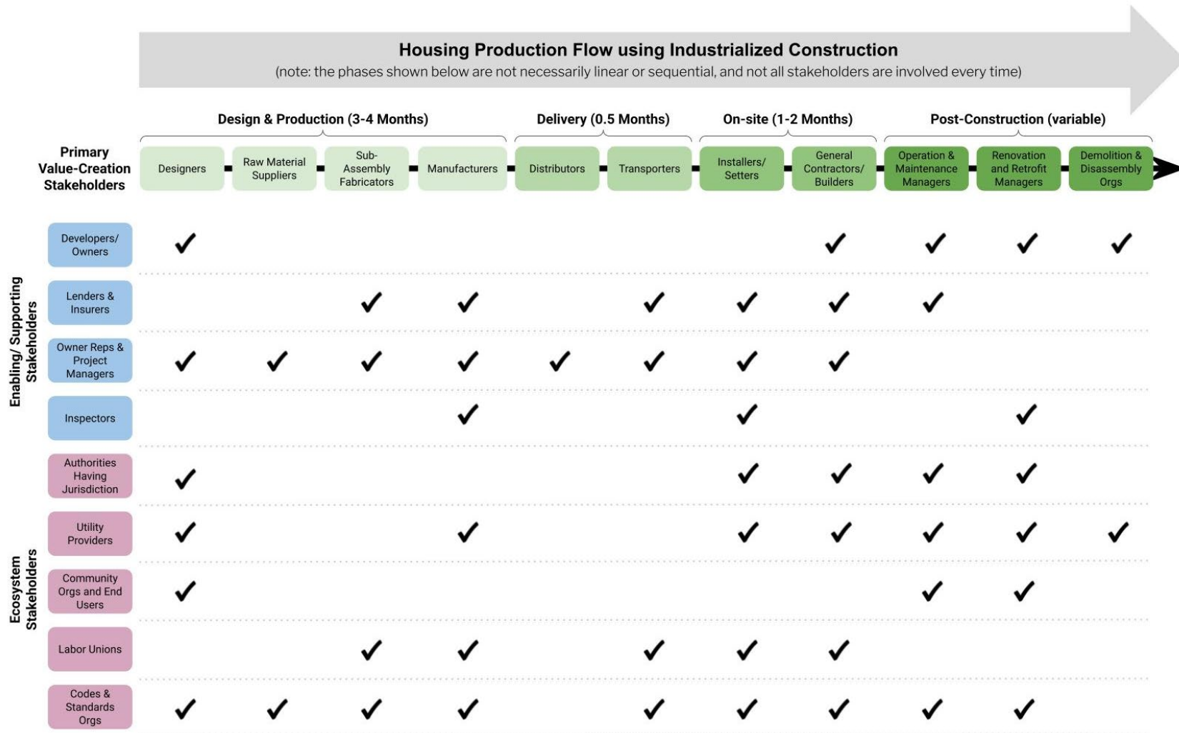
Fig. 4. Generalized IC housing production flow depicting value-creating stakeholders (green) and influencing stakeholders (blue and purple). Check marks indicate where influencing stakeholders exert direct influence on the value-creating stakeholders.
