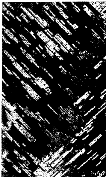
Fig. 25. STM image of a Si (001) surface following deposition of 0.1 monolayer Si at 580 K. Monolayer islands elongated along the dimer row direction for each terrace on the surface are clearly visible (from Ref. [205]).
