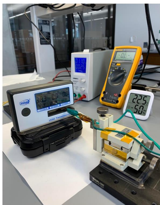
Figure S6. Experimental setup for transmittance-time response to the TC-PVK smart windows integrated with ZnO/Au/Al 2 O 3 TF, ZnO/Au/Al 2 O 3 NM and ITO glass.
