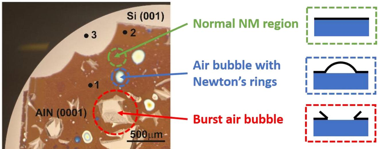
**Figure S4.** Optical image of the transferred AlN NM on the Si substrate with schematic illustration of various regions of the transferred NM. The sample has been annealed at 350 °C for 5 min in N<sub>2</sub> ambient via rapid thermal annealing (RTA) after the NM transfer.
