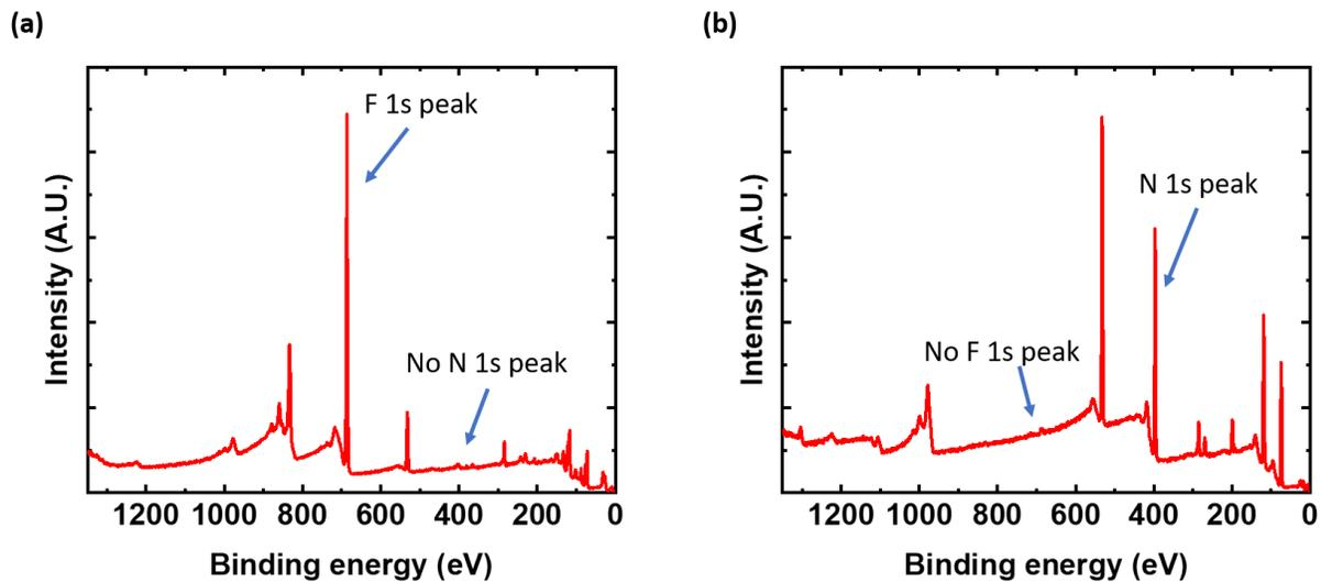
**Figure S2.** XPS survey spectra of the sample surface (a) right before Al removal and (b) after Al removal via RIE. The appearance of N 1s peak in (b) indicates that the AlN is exposed. Meanwhile F residue from the XeF<sub>2</sub> etching is observed in (a). And it can be removed by the RIE etching of Al.
