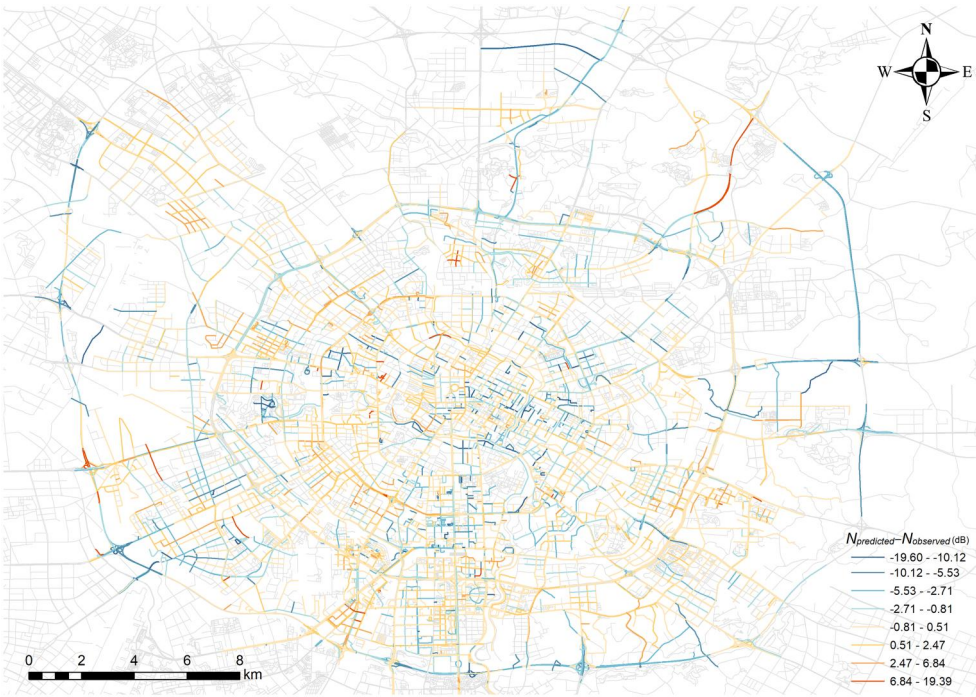
Figure A2. Difference map between the observed and the predicted road traffic noise within the outer ring freeway of Chengdu.
