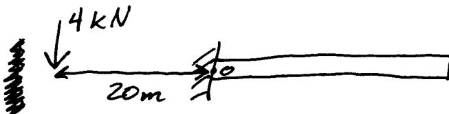
The resultant does not necessarily act at a point on the structure.
