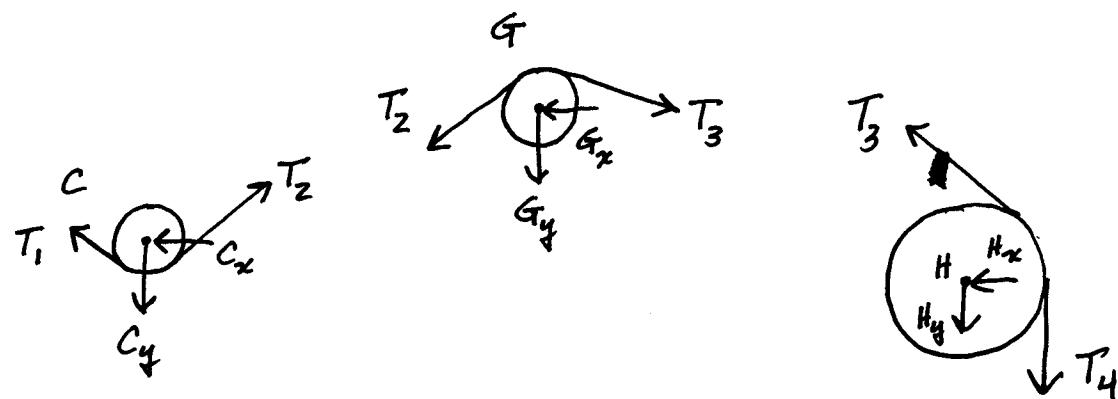
All internal forces come in equal but opposite pairs on the corresponding component FBDs. When you "add" all of the component FBDs.
