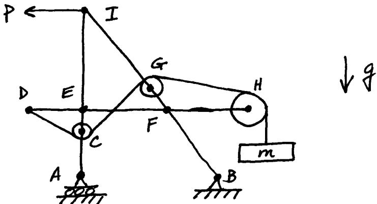
Bars IA, DH and IB are solid and joined together at E, I and F by frictionless pins. Weightless pulleys are attached at C, G and H by frictionless pins. Draw FBDs of the entire structure and each component of the structure.
