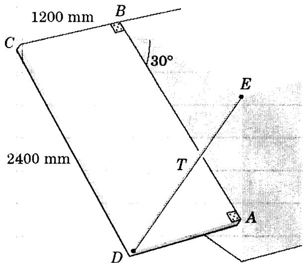
The uniform rectangular panel  $ABCD$  has a mass of 40 kg and is hinged at its corners  $A$  and  $B$  to the fixed vertical surface. A wire from  $E$  to  $D$  keeps edges  $BC$  and  $AD$  horizontal. Hinge  $A$  can support thrust along the hinge axis  $AB$ , whereas hinge  $B$  supports force normal to the hinge axis only. Find the tension  $T$  in the wire and the magnitude of the force supported by hinge  $B$ . ( $BEA$  is a right triangle.)
