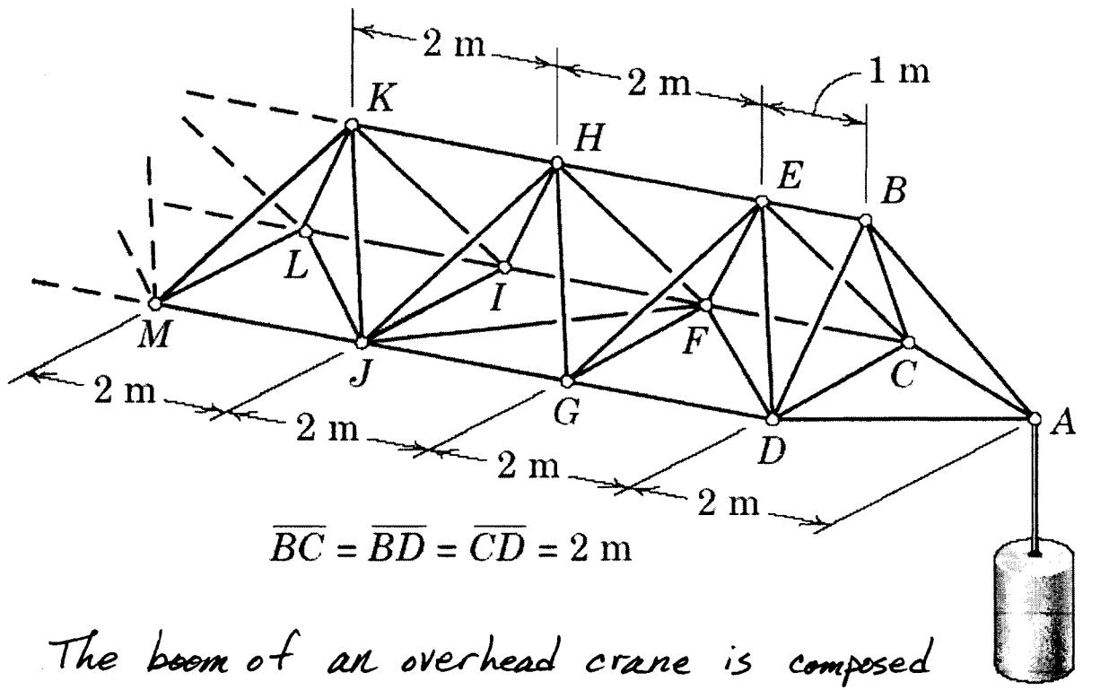
The boom of an overhead crane is composed of repeated and identical structural units. Use the method of sections to find the forces in members FJ and GJ.
