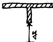
$$Q(y) = b \int_{h_1/2}^{h/2} y' dy' + t \int_y^{h_1/2} y' dy'$$
