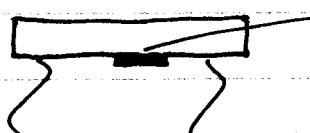
Here  $\tau \neq 0$  because there is material on the other side of the cut applying load.
