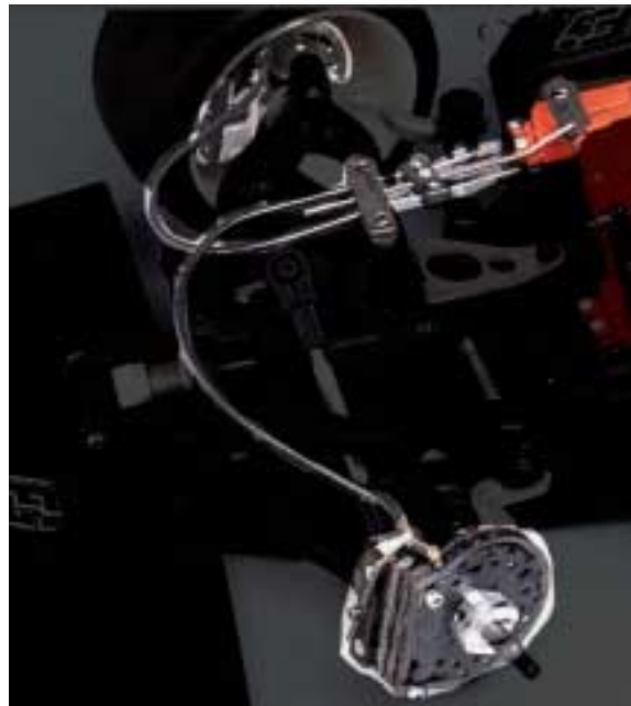
Figure 2.4 FGM Cable Actuated Brakes (highlighted for viewing)
