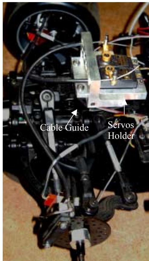
Figure 2.5 Modified Brake System Setup
