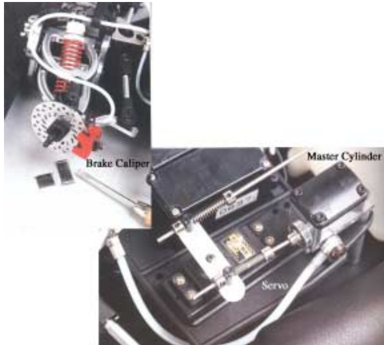
Figure 2.3 FGM Hydraulic Brake System
