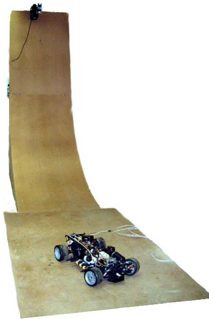
Figure 2.4 Test Platform – Test Track, Test Vehicle and Real-Time Controller [30]
