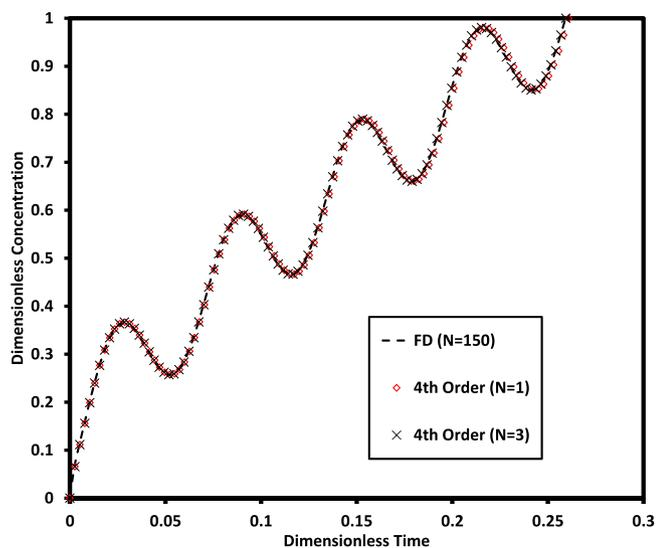
**Figure 3.** Comparison of Lobatto IIIA 4<sup>th</sup> order method with Finite Difference with constant diffusion coefficient and time dependent charging current.
