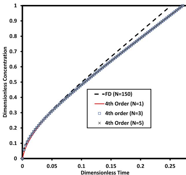
**Figure 4.** Comparison of Lobatto IIIA 4<sup>th</sup> order method with Finite Difference with concentration dependent diffusion coefficient and galvanostatic charging current.
