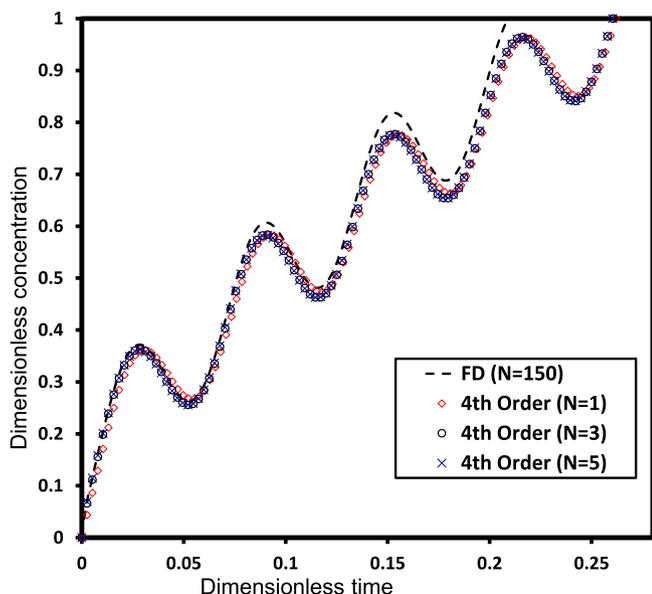
**Figure 6.** Comparison of Lobatto IIIA 4<sup>th</sup> order method with Finite Difference with concentration dependent diffusion coefficient and time dependent charging current.
