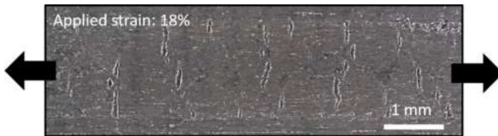
Figure S8. A global view of a Gr/PMMA ribbon on a 3M Tegaderm tape at fracture (18% of applied strain). Many macro-cracks transverse to the stretching direction are visible.
