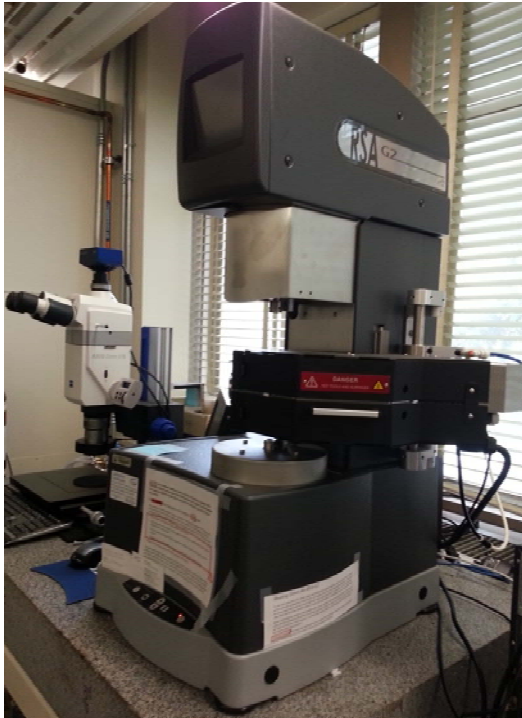
Figure 14: Experimental Apparatus: Zeiss microscope and RSA G2, DMA.
