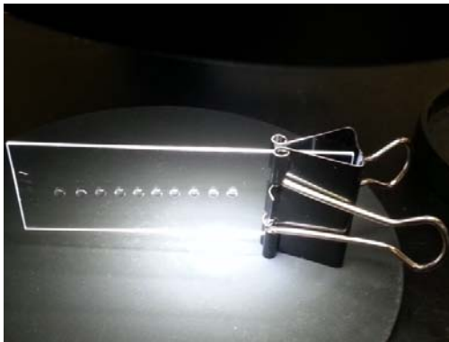
Figure 16: PDMS lens on a glass slide observed under a microscope from the side view.
