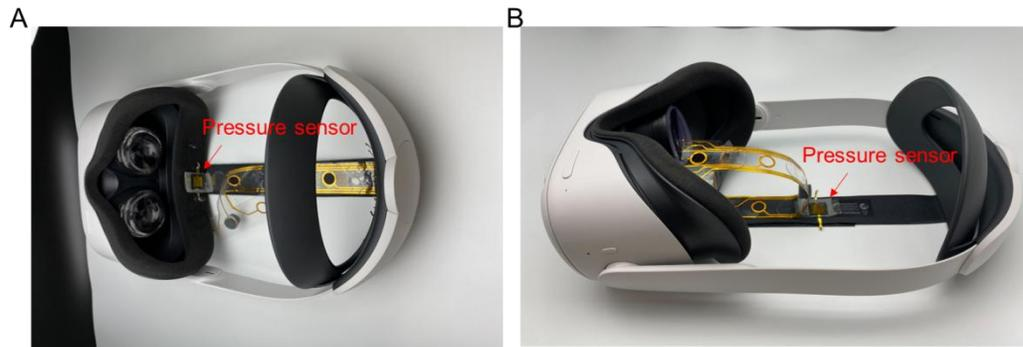
Figure 6. The setup used in measuring the pressure exerted by the VR headset strap on the hairless site (A) and on the hairy site (B).
