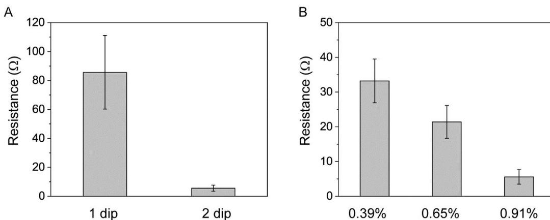
**Figure 4.** Resistance of the PMA sponges prepared with different parameters. (A) Comparison of the PMA sponges with different dipping cycles ( $n = 12$ ). (B) Comparison of the PMA sponges prepared in PEDOT:PSS solution with different PEDOT:PSS concentrations ( $n = 12$ ).
