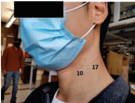
Figure 7 | In vivo placements of the e-tattoo on the neck. PPG signals were obtained from different locations on the neck to observe the changes in waveform morphology.
